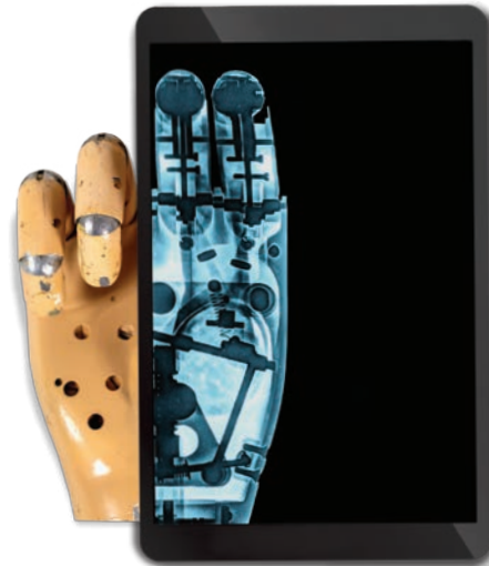
"Belgrade hand" Revealing its secrets through advanced radiology techniques (dynamic imaging) The world's first robot hand from 1963 gets a new life made in the European congress of radiology in Vienna 2022.
